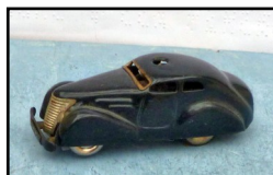
Schuco clockwork-driven auto-steering Car
